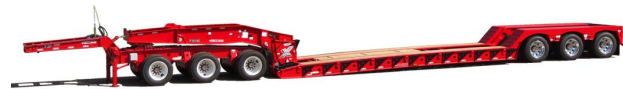
Shown with optional XF-Jeep 80-3, flip neck, outrigger boards w/hold downs & alum. wheels.
